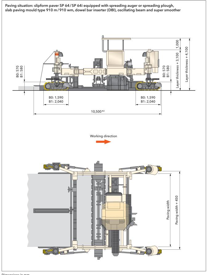
Dimensions in mm \*<sup>2</sup> = Applies to standard longitudinal joint tie bar inserter (non-pivotable)
