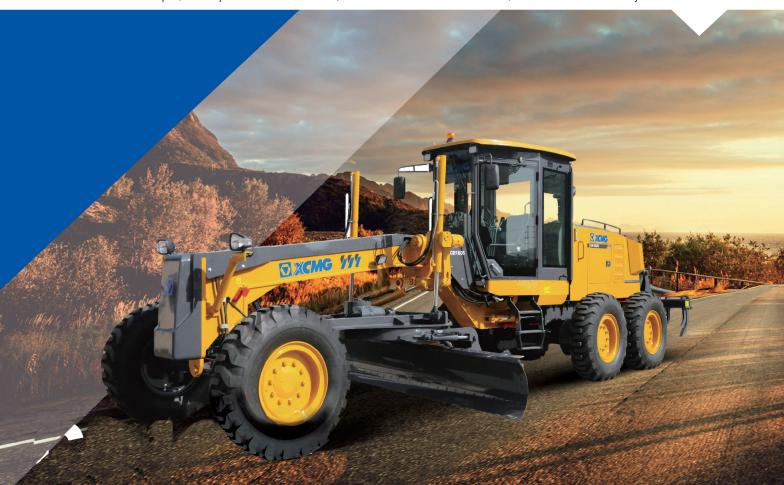
GR 1605 is mainly used for large ground surface leveling, ditching, slope scraping, bulldozing, scarifying, snow removing and other work in highway, airport and farmland. The grader is necessary engineering machinery for national defense construction, mine construction, urban and rural road construction, water conservancy construction and farmland improvement, etc
