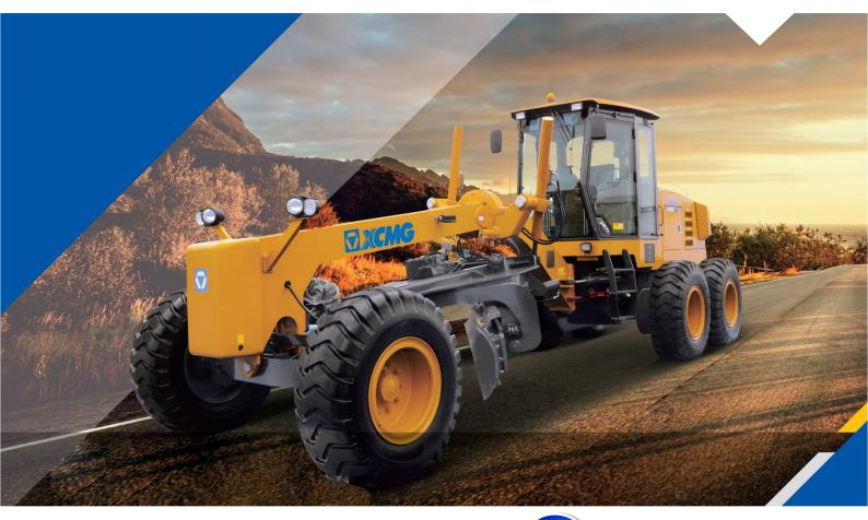
GR 2403 is mainly used for large ground surface leveling, ditching, slope scraping, bulldozing, scarifying, snow removal for large areas such as highway, airports, farmlands etc. It is the necessary construction machinery for national defense construction, mine construction, urban and rural roads, and mine roads construction and water conservancy construction, farmland improvement and so on.
