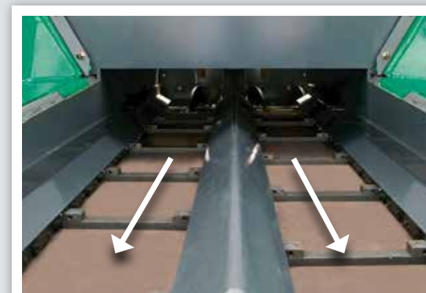
CONVEYOR MOVEMENT REVERSIBLE FOR A SHORT TIME
