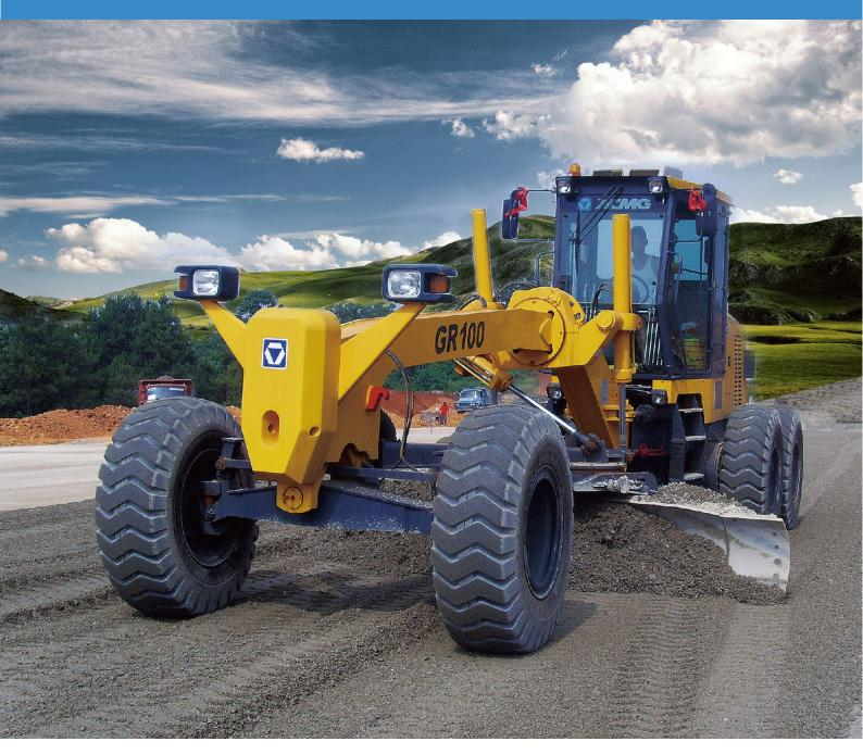
The XCMG GR100 motor graders are primarily comitted to operations as ground leveling, trenching, cutting surface, dozing, soil loosening and snow plowing of roads, airports, farmlands and others. They are the exclusive and needful construction machinery for national defense engineering, mine construction, building of town and country roads, water conservancy construction, farmland improvement and etc
